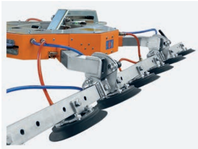
The steplessly variable suction pad adapter allows suctioning convexly and concavely curved panes with radii \geq 1.0 m.
